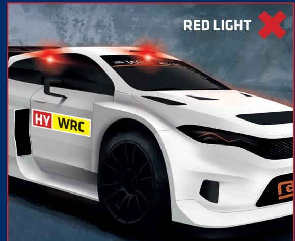
**3** A flashing red light, along with an alarm sound, means the car is unsafe. No light means it is potentially unsafe. Only touch the car if there is a green light.
