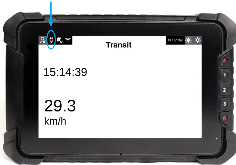
Figure 1 - White power light: device powered correctly
