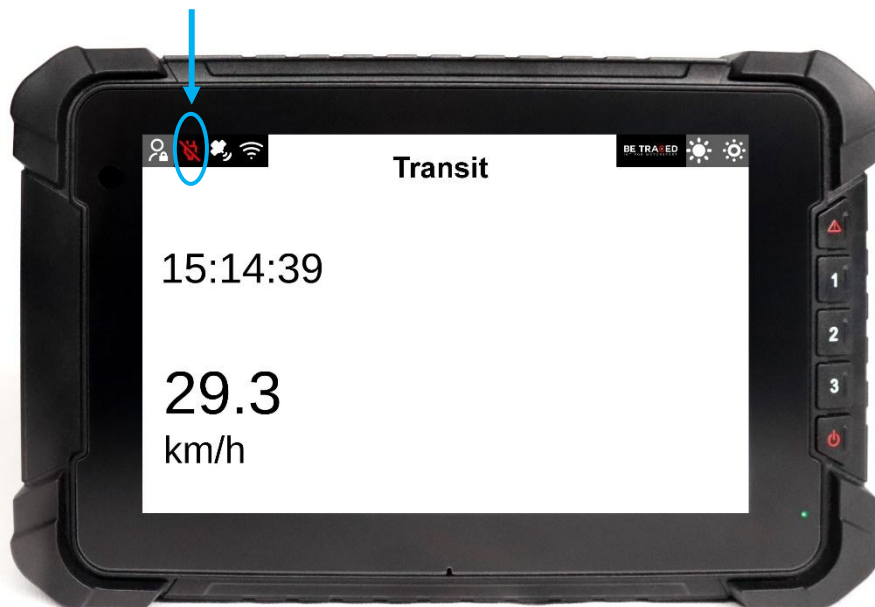
Figure 2 - Red power indicator light: device not powered
