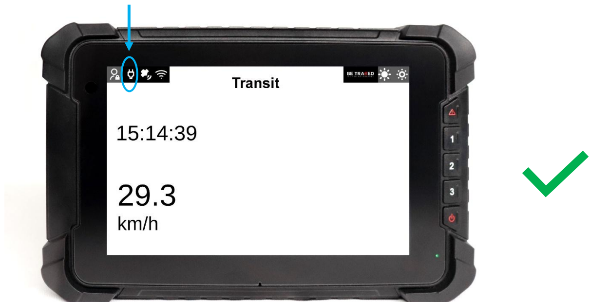
Figure 1 - White power light: device powered correctly
