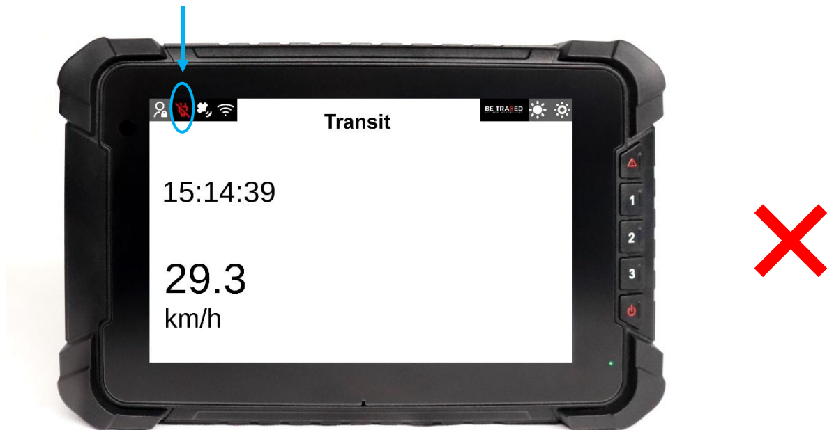
Figure 2 - Red power indicator light: device not powered
